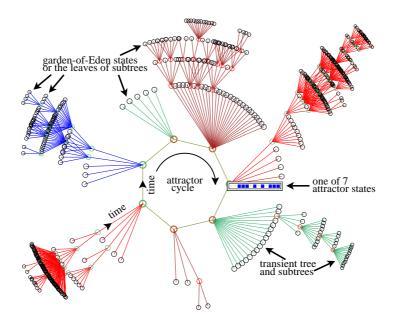
Fig. 6: A basin of attraction (one of 15) of the RBN (n=13, k=3) shown in figure 5. The basin links 604 states, of which 523 are garden-of-Eden states. The attractor period = 7, and one of the attractor states is shown in detail as a bit pattern. The direction of time is inwards from garden-of-Eden states to the attractor, then clock-wise. [0.56sec]
