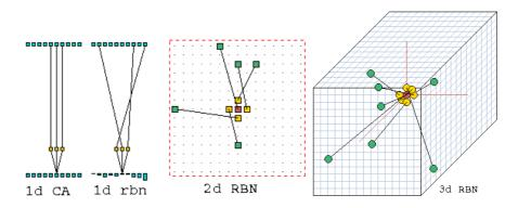
Fig. 22: The wiring of a cell: for random wiring, cells anywhere in the network are wired back to each position in a "pseudo-neighborhood," which corresponds to the CA neighborhood. Each cell's wiring can be shown (and amended) by moving around the network with the mouse or keyboard. *Left:* 1D: The wiring is shown between two time-steps. *Center:* 2D: k=5. *Right:* 3D: k=7.
