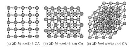
Fig. 2: Network-graphs of: (a) A small 2D CA, (b) a 2D CA on a hexagonal lattice, (c) a 3D CA. These network-graphs can be created and manipulated in DDLab.
