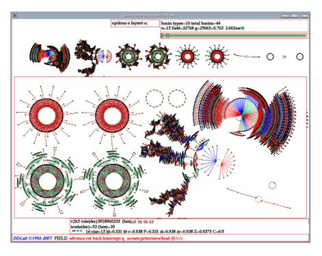
Fig. 31: The DDLab screen showing two layouts of a basin of attraction field. Top: the normal layout but with spacing adjusted after each basin. Inset below: the layout-graph where nodes (thus basins) can be dragged into any position. Both results can be saved as vector PostScript files. This example is for a binary 1D CA, k=5, totalistic rule 53, n=15 [2.4 sec].
