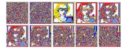
Fig. 43: To decrypt, starting from the encrypted state in Fig. 42, the CA with the same chain-rule was run forward to recover the original image. This figure shows time steps -2 to +7, to illustrate how the portrait was scrambled both before and after time-step 4
