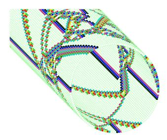
Fig. 9: A 1D space-time pattern shown as a ring of cells. scrolling diagonally towards the top left. The present moment is the ring at the bottom right. The space-time pattern is colored according to neighborhood, and has been filtered. 1D binary CA, k=5, hex rule e9 f6 as 15, n=150 (as in Fig.16).
