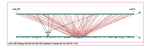
Fig. 26: The 1D wiring graphic, showing wiring to a block within a 1D network. k=5, n = 150. The block was defined from cells 60–80. Revisions to rules and wiring can be the confined just to the block. The "active cell" is still visible and can be moved as usual. The 1D wiring graphic can also be shown as a circle.
