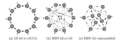
Fig. 1: Network-graphs of: (a) The simplest 1D CA, n=10 cells and k=3 inputs per cell, one from each neighbor and one from itself. Periodic boundary conditions make the cells form a ring. Wolfram called these "elementary" CA [13]. (b) n=10, k=3 RBN wired at random, and (c) the same RBN unscrambled – nodes rearranged.
