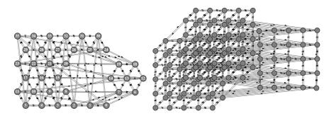
Fig. 28: Network-graphs of a 2D and 3D CA. *Left*: a 2D hexagonal network, showing a node and its 1-step inputs dragged out. *Right*: a 3D network shown as an axonometric projection seen from below as if looking up into a cage. A vertical slice has been defined and dragged from the graph.
