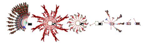
Fig. 10: basin of attraction field of a 3-value Cellular Automaton, [v, k, n] = [3,3,8], rule 020120122021201201011011022. There are in fact 17 basins, but equivalent basins have been suppressed leaving just the 7 prototypes. One attractor state is shown for each basin [0.16sec].
